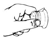
First make sure knobs are on OFF then pull knob straight off.
